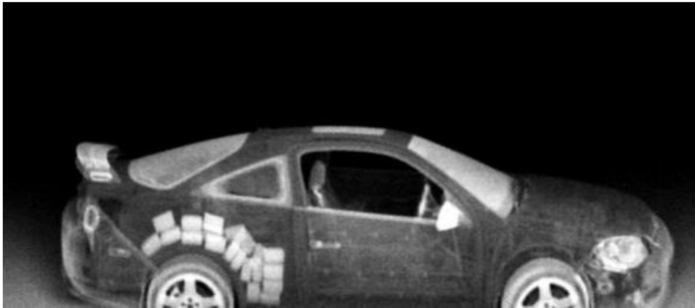
Figure 9: Example of non-intrusive inspection technology image
